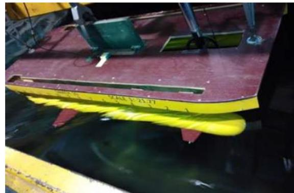
Fig.10: Experimental setup with fins attached to hull different speed
