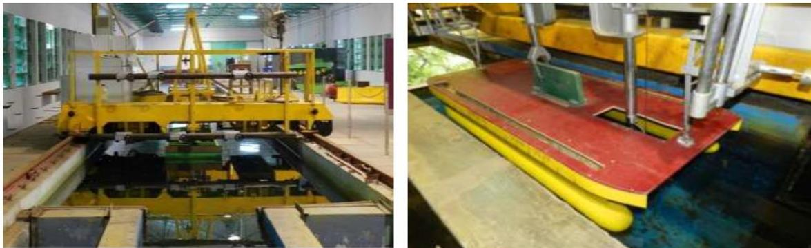
Fig.7: Experimental setup for drag test
